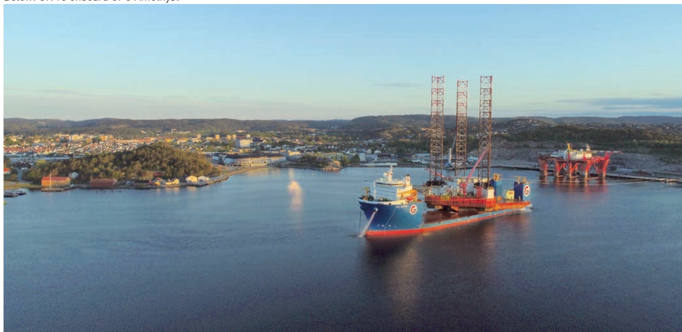
Above: Float over of UR 93 to GPO Amethyst Below: UR 93 onboard GPO Amethyst
